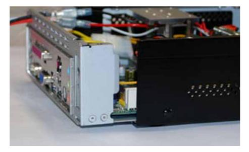
Now connect the HDD with the adapter SATA-HDD 2,5" to SATA-MB and power, it is only possible to connect in one direction.
