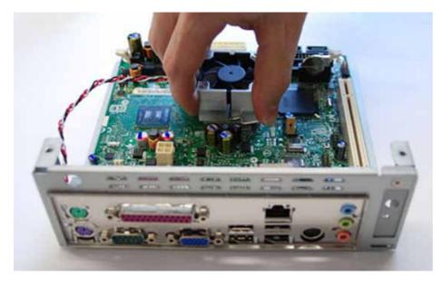
Clean the CPU (marked) and the chipset (marked).
