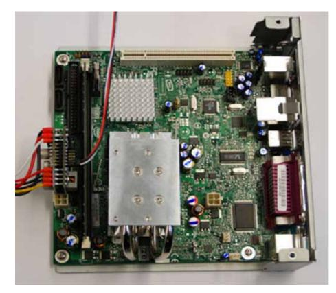
Please connect the switch cable of the remote cable from your M3-ATX adapter with the red marked PINs (according to Intel) right next to the power LED plug.
