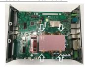
8. Fix CPU heat-sink by M3 screws(x 4, pack 452D80500002) as arrow shown.
