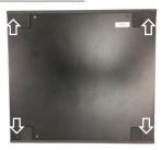
1. Loosen M3 screws(x 4) from Bottom cover as the arrow locations.
