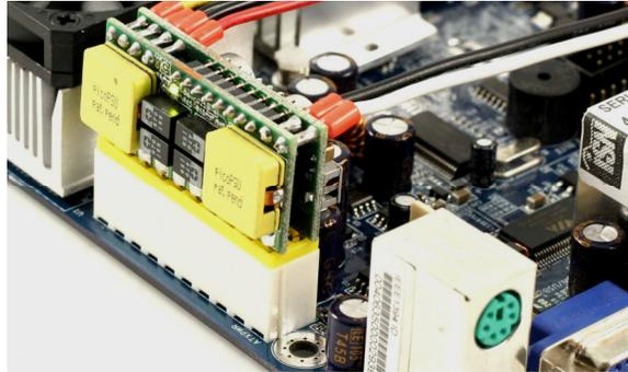
*Fig 1.1 picoPSU-150-XT plugged into ATX connector.*
